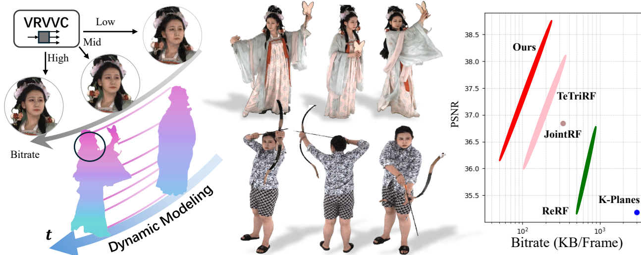
Figure 1: Left: Our proposed VRVVC efficiently compresses volumetric video at variable bitrates using a single model. Middle: We demonstrate two examples of reconstruction quality at a bitrate of 60 KB per frame. Right: The RD performance of our approach surpasses prior work (e.g. ReRF (Wang et al. 2023), TeTriRF (Wu et al. 2024))
