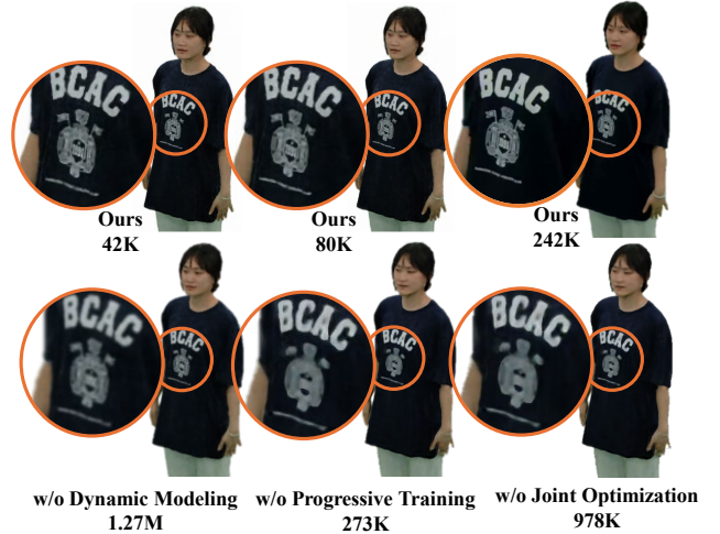
Figure 7: Qualitative results of complete VRVVC and its variants. Excluding any module results in lower reconstruction quality and an increase in bitrate.
